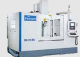
▲ 1270-H3L • Travel : X1200 Y700 Z650 mm • Table : L1350×W600 mm
