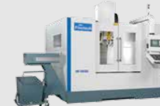
▲ 1060-H3L • Travel : X1000 Y600 Z560 mm • Table : L1100×W500 mm
