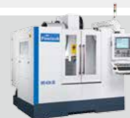
▲ 1060-2LB/3B • Travel : X1000 Y600 Z560 mm • Table : L1100×W500 mm
